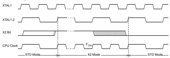
The X2 bit in the CKCON0 register (see Table 16) allows a switch from 12 clock periods per instruction to 6 clock periods and vice versa. At reset, the speed is set according to X2 bit of Hardware Security Byte (HSB). By default, Standard mode is active. Setting the X2 bit activates the X2 feature (X2 mode).
