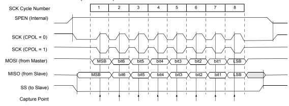
Figure 33. Data Transmission Format (CPHA = 1)
