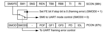
When this feature is enabled, the receiver checks each incoming data frame for a valid stop bit. An invalid stop bit may result from noise on the serial lines or from simultaneous transmission by two CPUs. If a valid stop bit is not found, the Framing Error bit (FE) in SCON register (See Table 33.) bit is set.
