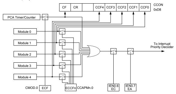
**PCA Modules:** each one of the five compare/capture modules has six possible functions. It can perform:
