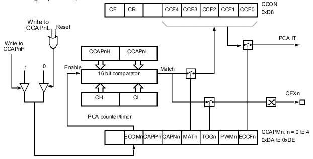
Before enabling ECOM bit, CCAPnL and CCAPnH should be set with a non zero value, otherwise an unwanted match could happen.
