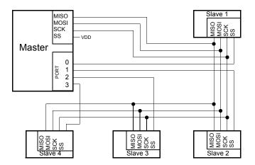
The Master device selects the individual Slave devices by using four pins of a parallel port to control the four SS pins of the Slave devices.
