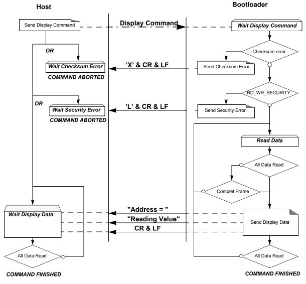
Note: The maximum size of block is 400h. To read more than 400h bytes, the Host must send a new command.
