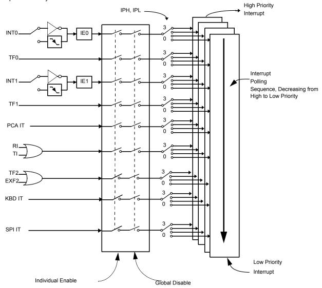
Each of the interrupt sources can be individually enabled or disabled by setting or clearing a bit in the Interrupt Enable register (Table 54 and Table 56). This register also contains a global disable bit, which must be cleared to disable all interrupts at once.
