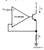
$I_O = 1 \text{ amp/volt } V_{IN}$ (Increase  $R_E$  for  $I_O$  small)
