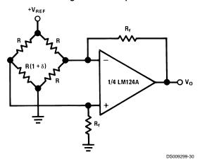
For  $\delta << 1$  and  $R_f >> R$   $V_O \cong V_{REF} \left(\frac{\delta}{2}\right) \frac{R_f}{R}$
